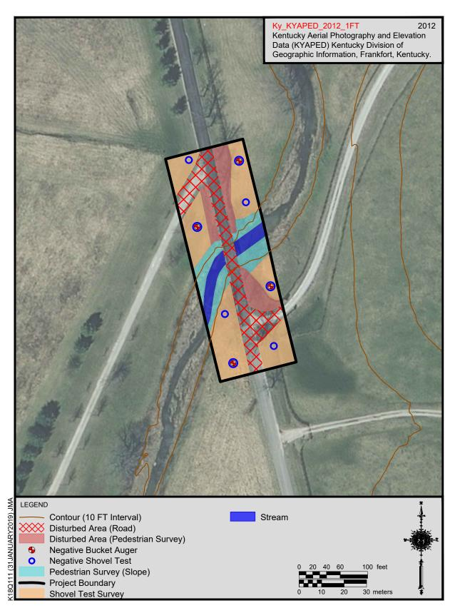
Figure 3. Project Area plan for the CR 1205 Bridge (009C00031N) over Houston Creek (Item No. 7-10007.00), Bourbon County, Kentucky.
